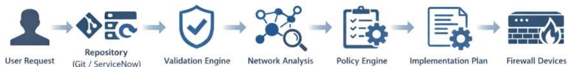
Fig. 1. Architecture of the automated firewall policy management system
